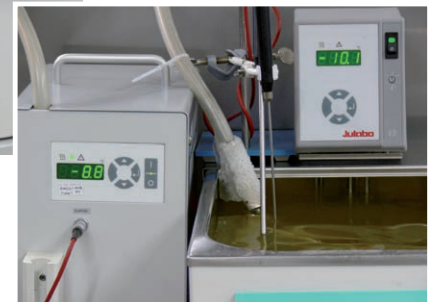
Setup with heating bath circulator and immersion cooler
