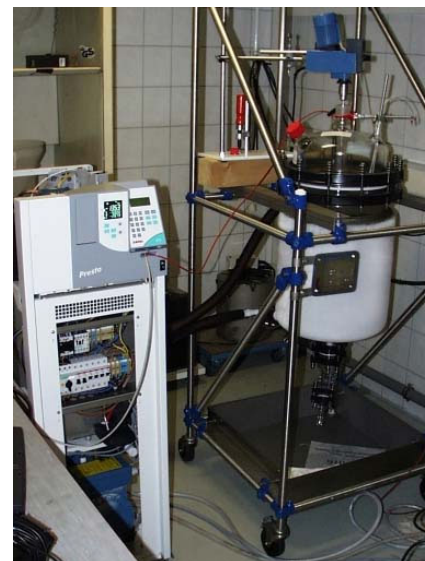
Overview of apparatus set-up. Notice the white frost surrounding reactor (far right) in test #2.
